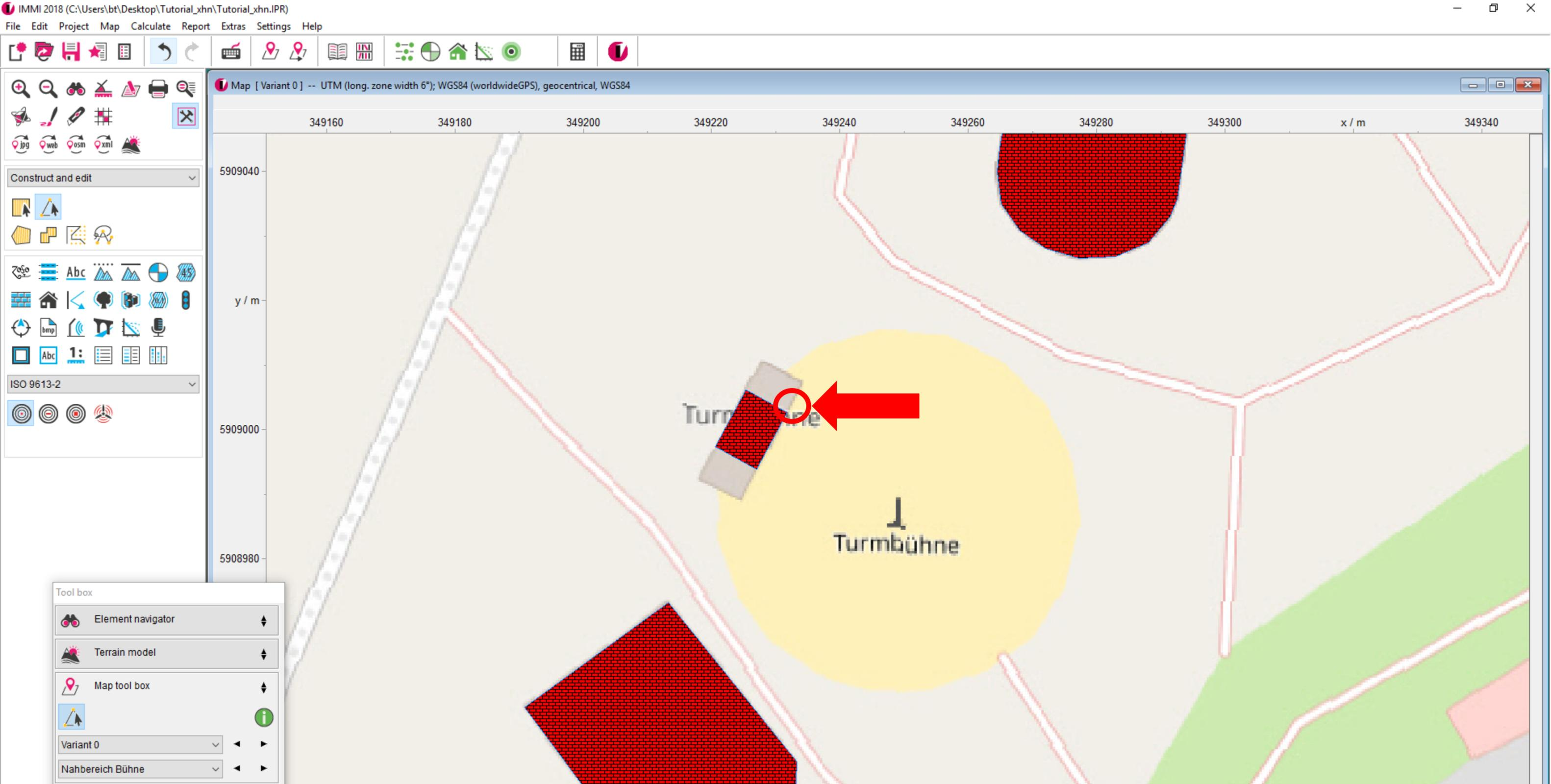
First we model the one on the left side of the stage. After clicking the position with left mouse button, the input dialogue opens.
