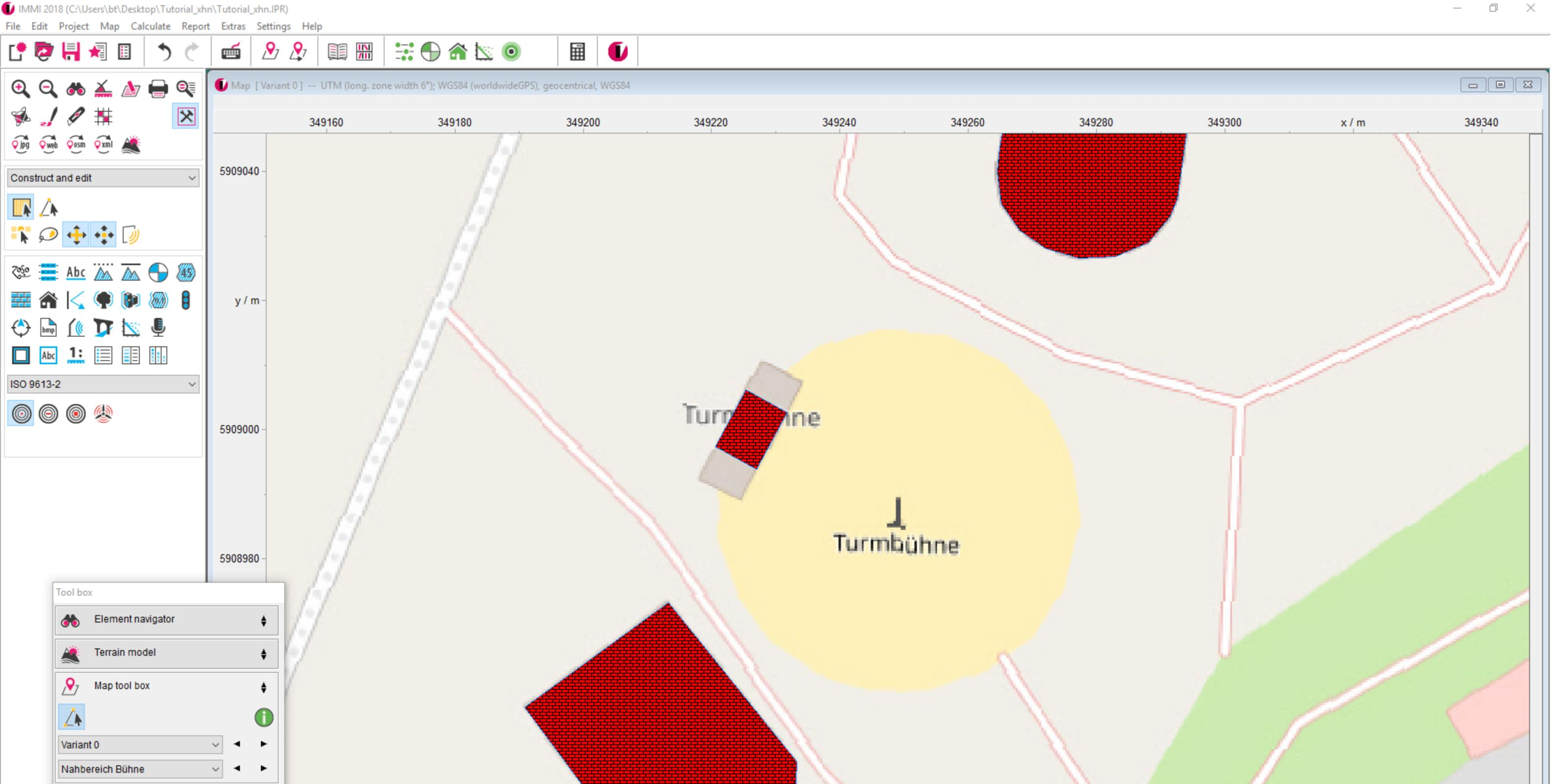
Back in the IMMI project, the first step is to model the line arrays as point sources according to ISO 9613-2 at the center stage.
