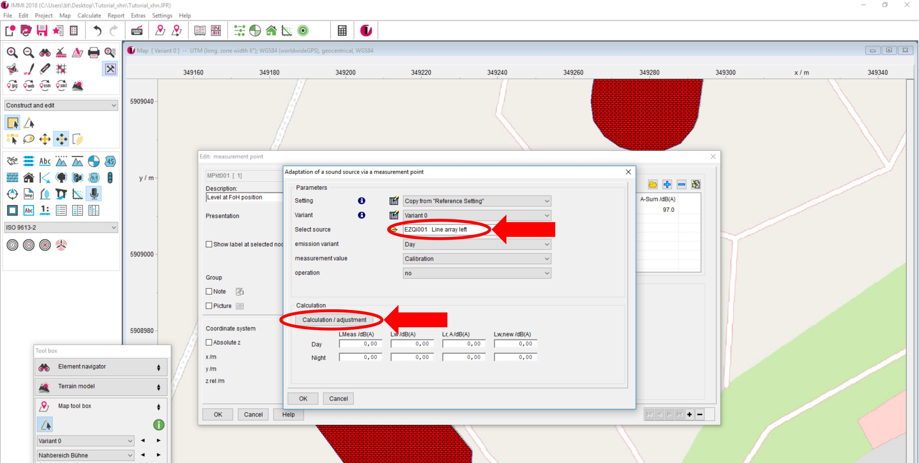
Make sure that „Line array left“ is selected and click „Calculation/adjustment“.
