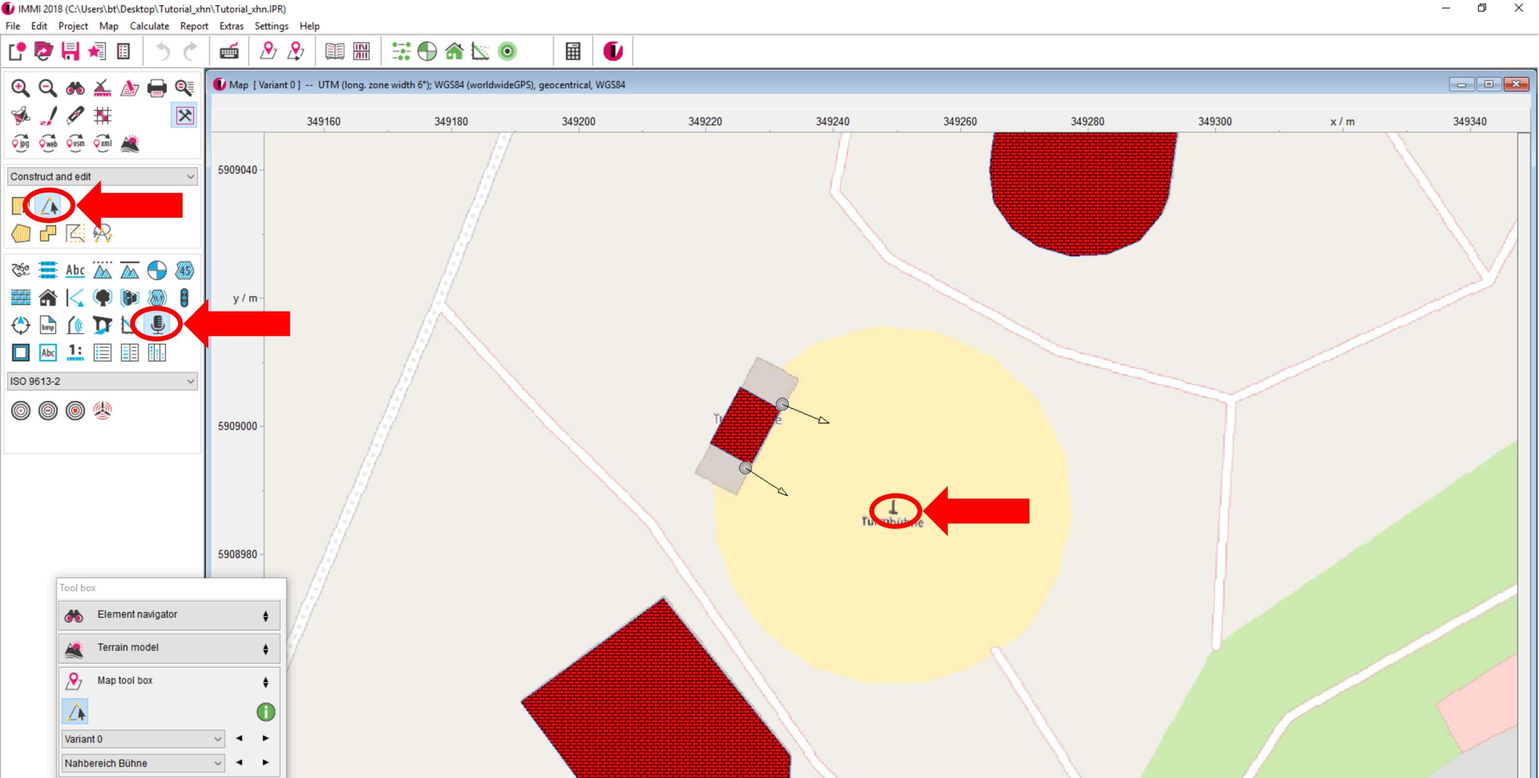
Please select the construction tool and the measurement point and model a measurement point at the center of the audience.
