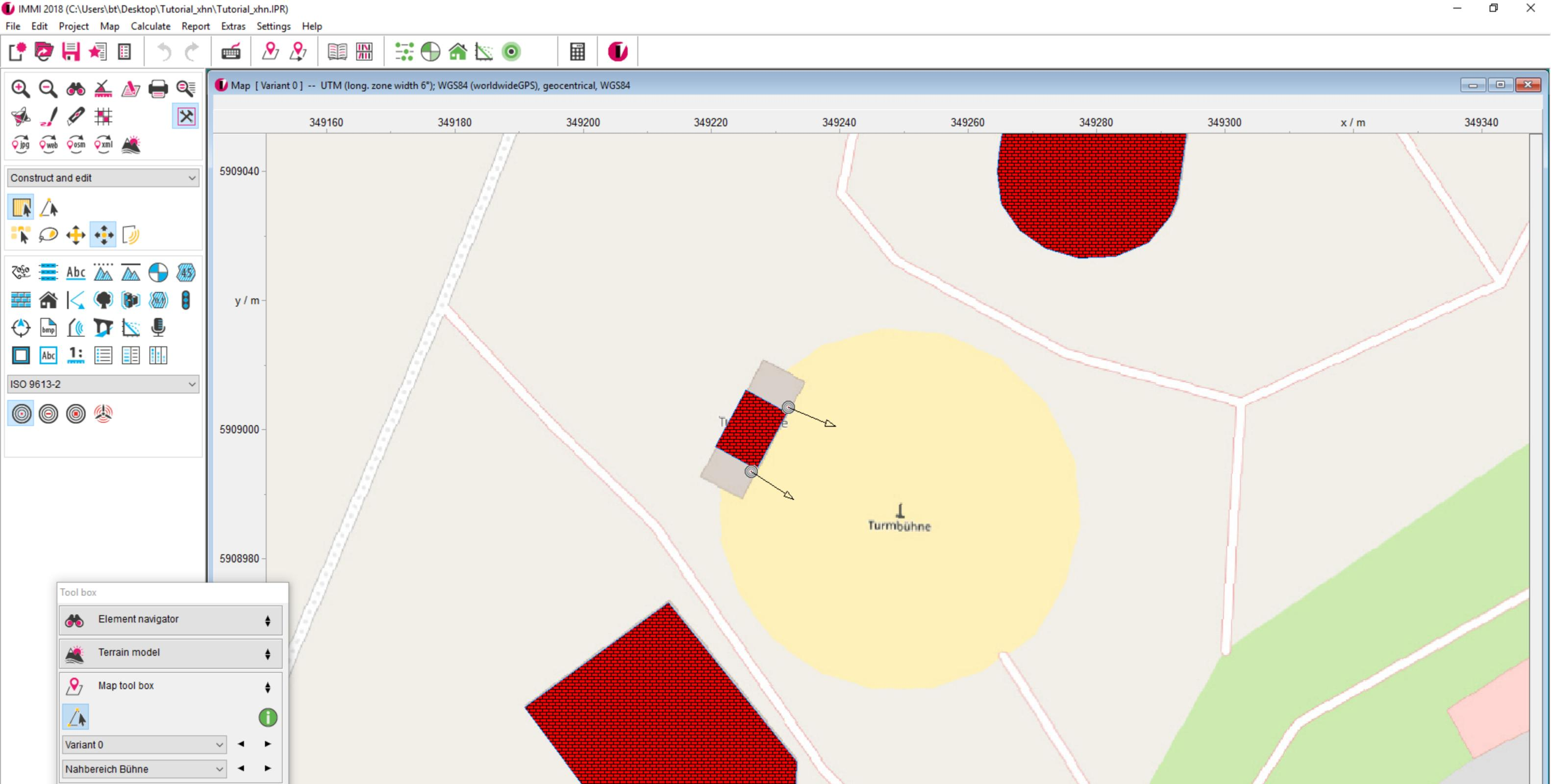
With this element we can calibrate the sound power level of the arrays to the desired value in the audience (FoH position).
