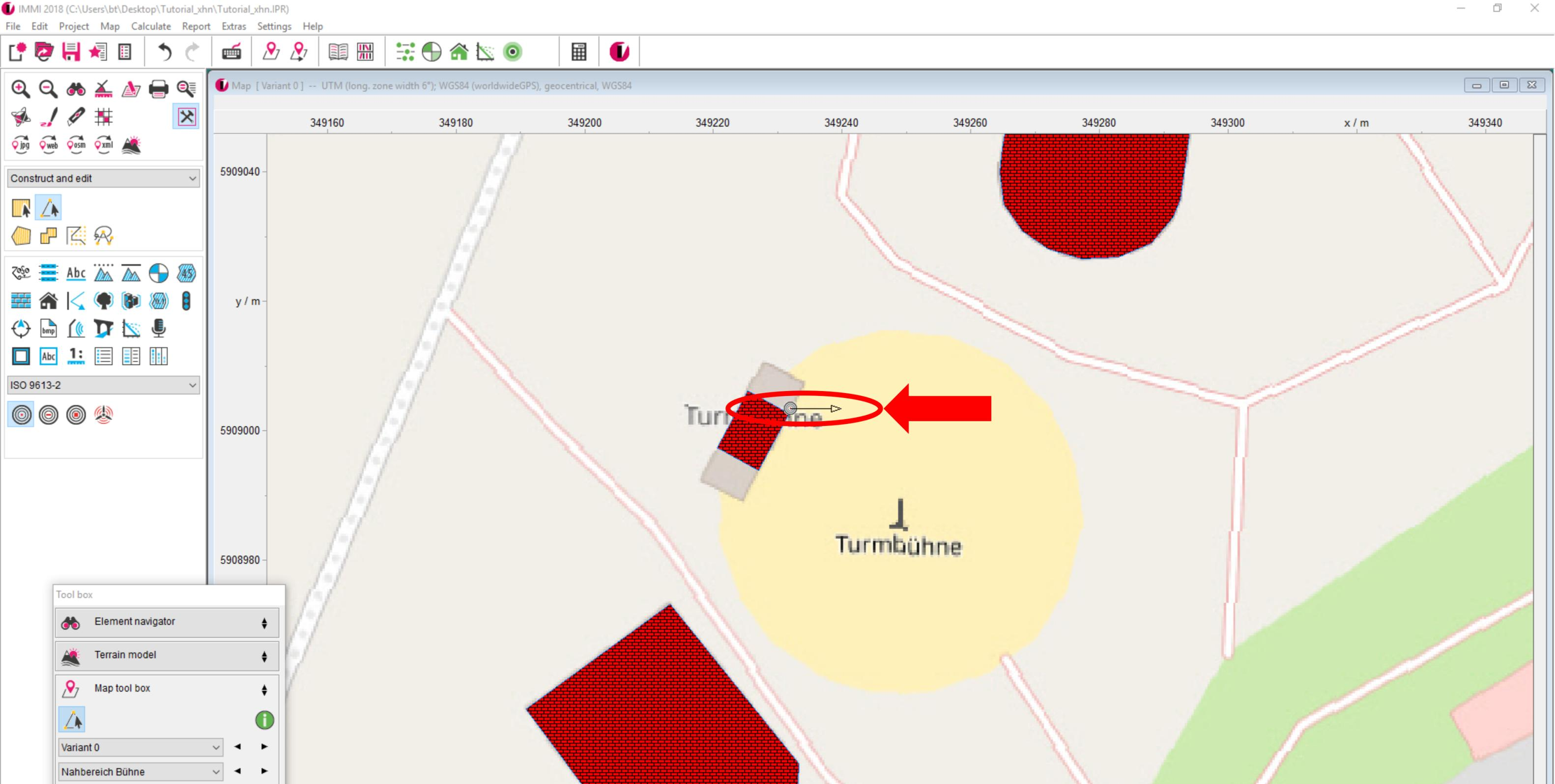
After closing the element dialogue with „OK“, the orientation of the directivity is displayed as a vector in the map.
