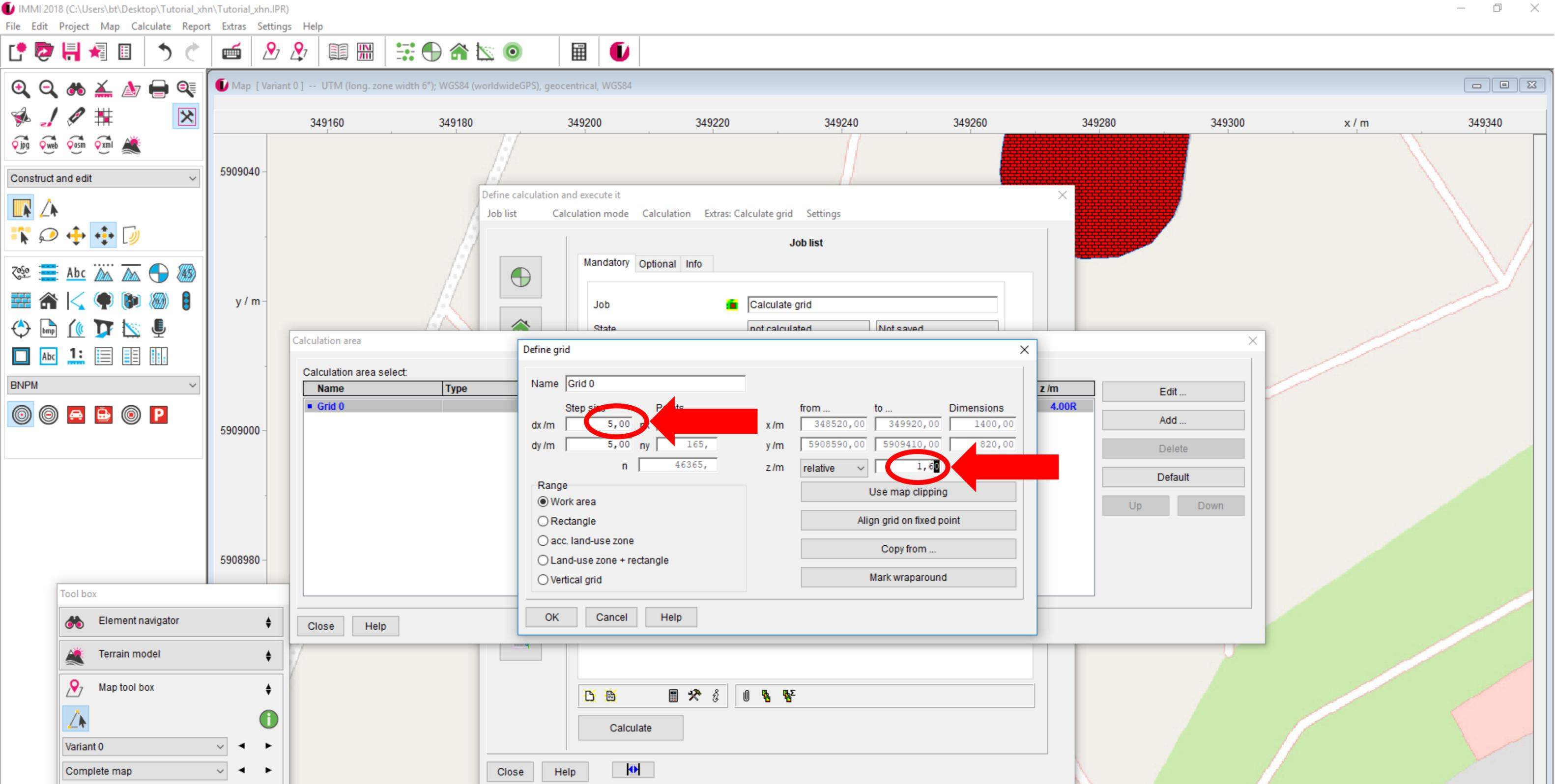
Change the step size in x and y direction to 5 m and set the relative height to 1,6 m.
