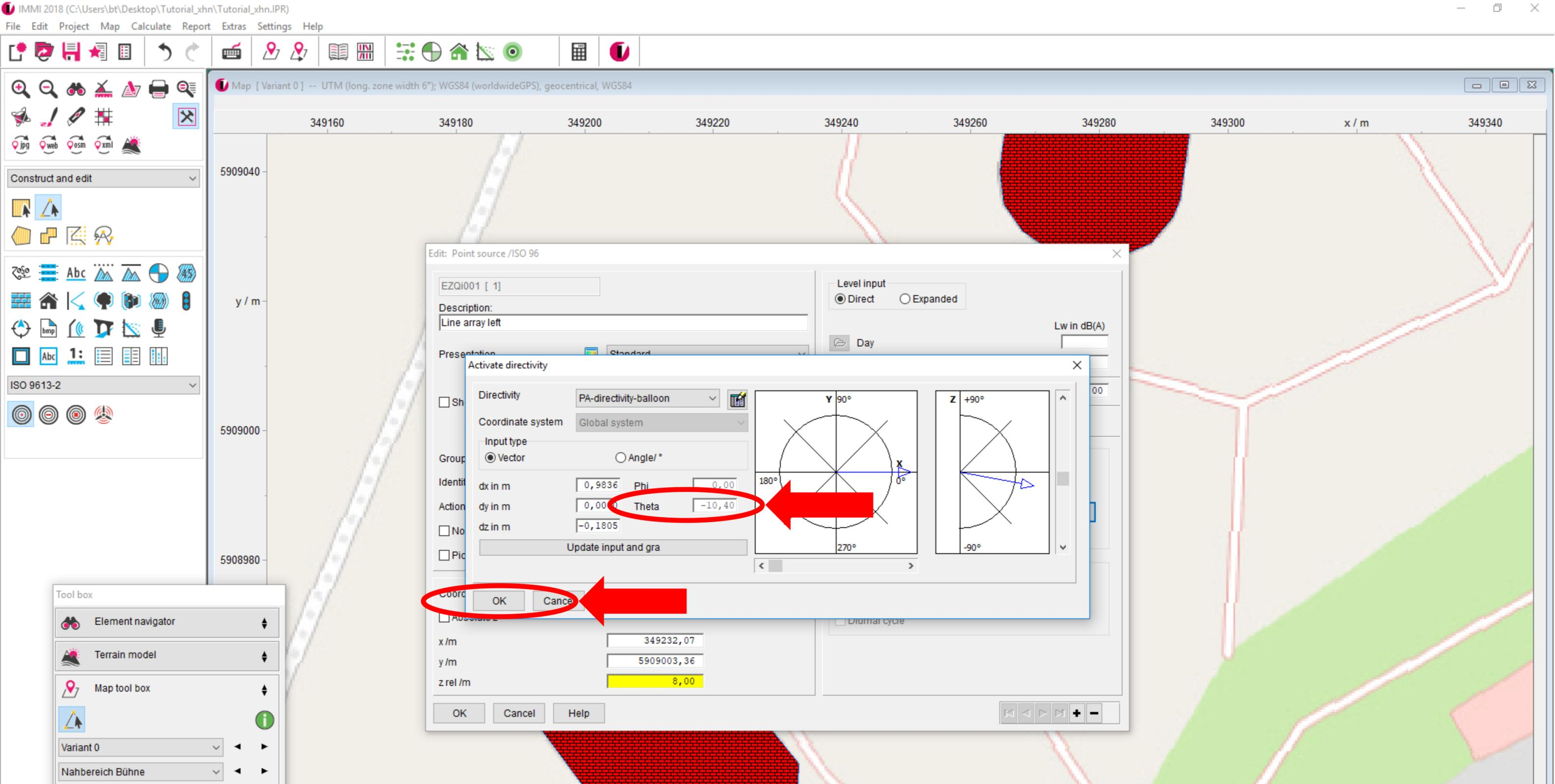
Enter the angle  $\alpha$  in the text field for „Theta“ in order to define the slight downward orientation of the array. Confirm with OK.
