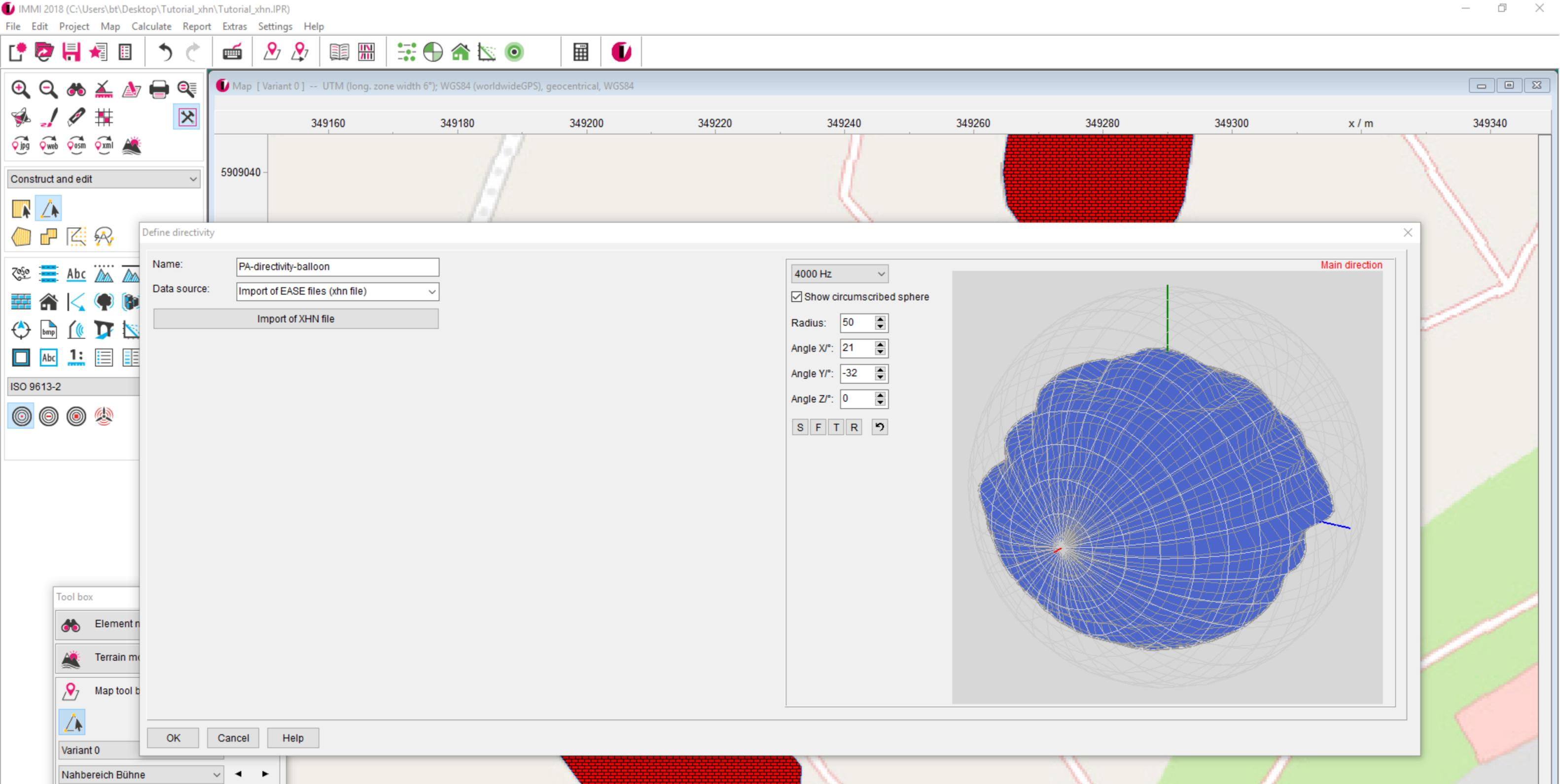
The balloon has been imported. You can now switch between the different frequencies and display different views.
