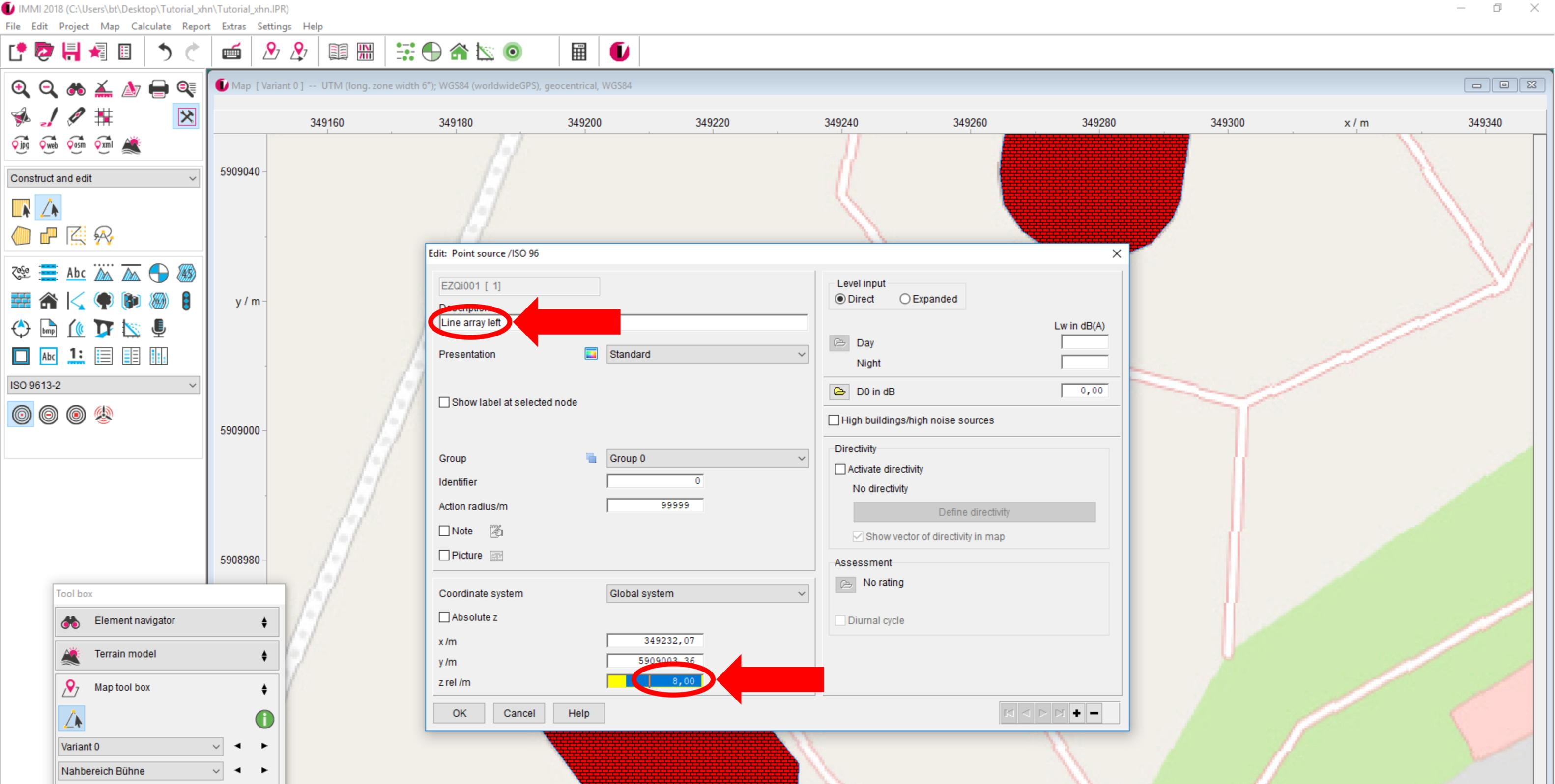
Type in the element name and set the value for the height according to the parameters from Soundvision.
