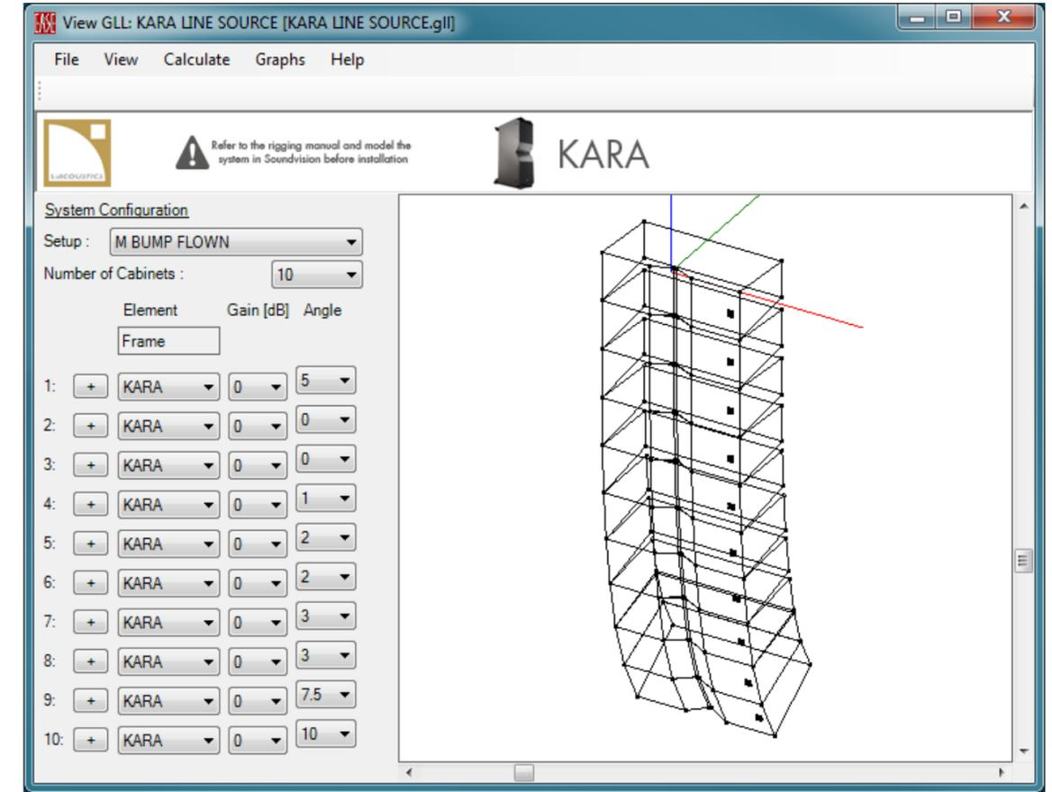
By introducing the parameters from Soundvision (see 3 slides before) to EASE Speaker Lab Pro, the complete setup is defined here.
