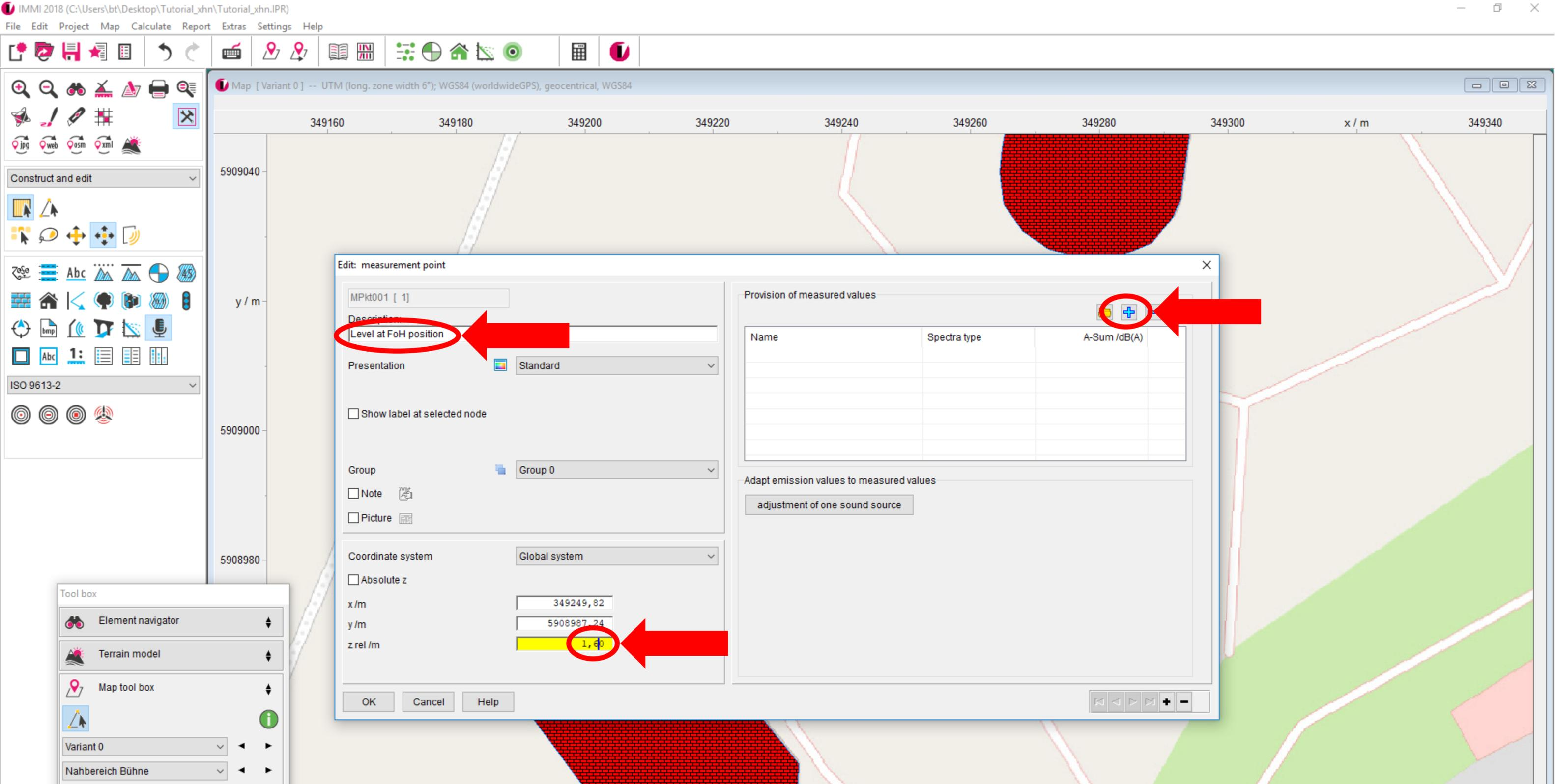
Enter a description and a relative height. Then press the „+“ button in order to define the level to which the line arrays shall be calibrated.
