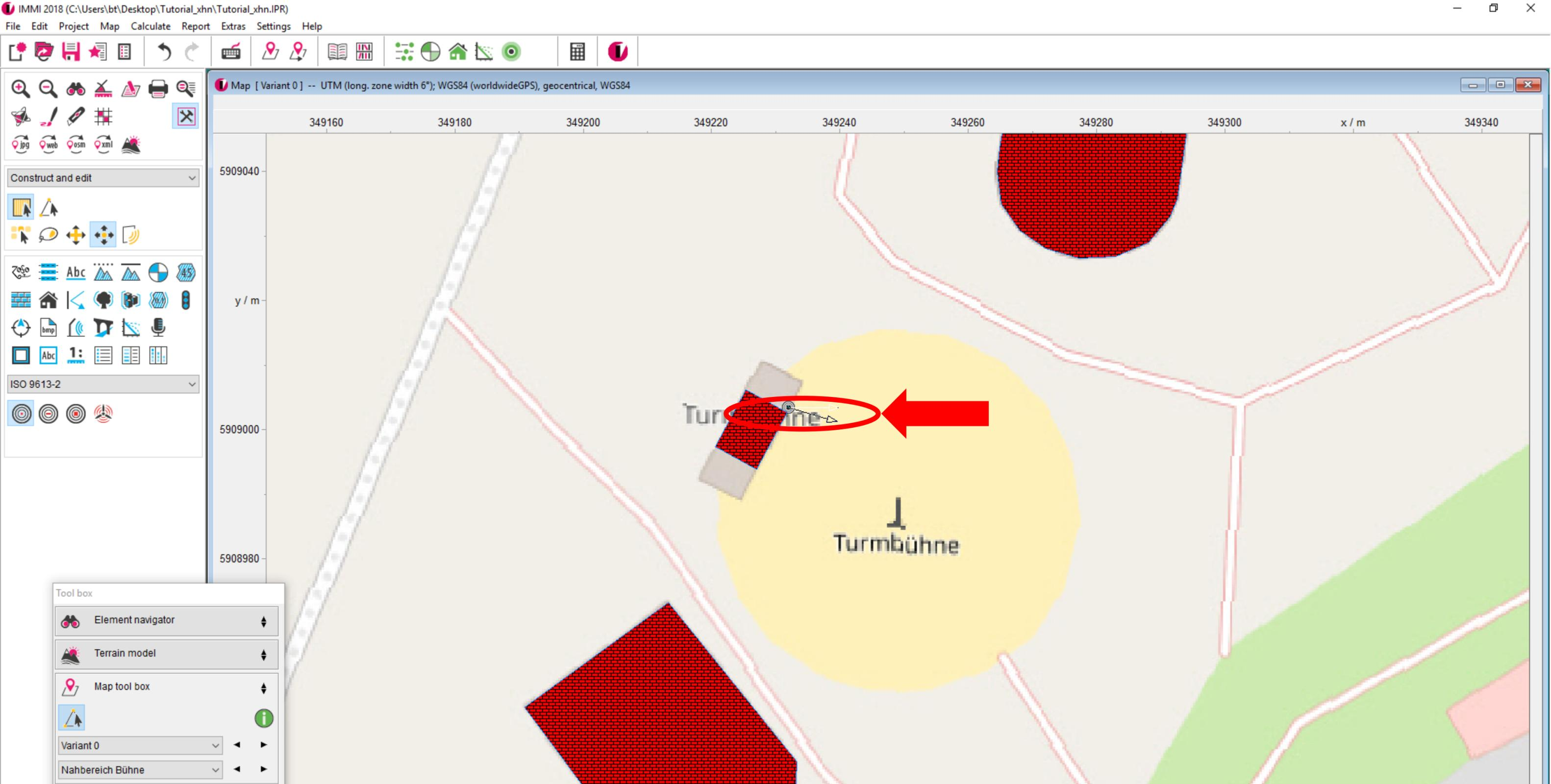
The directivity can be rotated by pressing the shift key, holding the left mouse button and moving the mouse.
